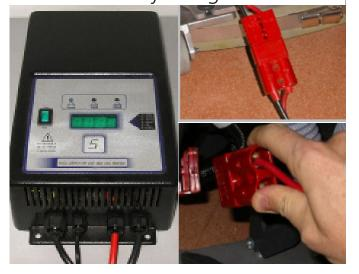
1a. Switch off charger by pressing the STOP button. Unplug charger cable from red battery plug. Reconnect the red battery plug to the machine.
