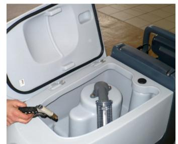
13. Wash with clean water the recovery tank and the vacuum grid.
