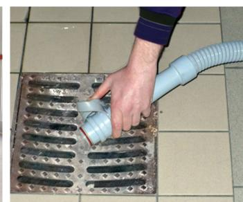
12. **At the end of the work.** Empty the recovery tank with the hose.
