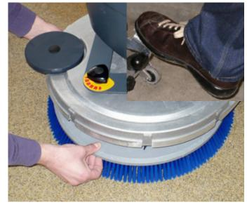
5. Place the brush or the pad-holder under the deck. Use the appropriate brush to clean the floor. Lower the deck by pressing the pedal deck.
