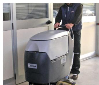
11. Push the drive paddle for starting floor cleaning. If solution applied flows outside the brush housing during use, reduce the flow of solution. Switch off the machine using the key.
