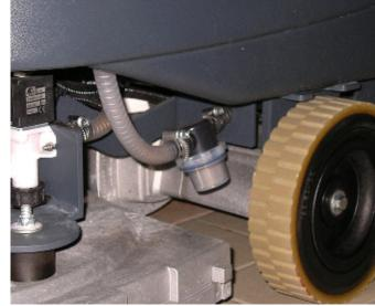
14. Clean the filter: 1) Close the solution tap under the machine. 2)
