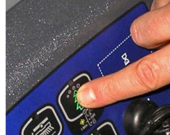
9. Press the EcoFlex<sup>™</sup> switch whenever you temporarily need a greater cleaning power.
