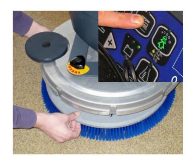
15. Press the switch and wait for the brush to fall on the floor.Remove the brush and clean them.
